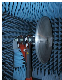
Figure 11. Rolled edge ground plane for GPS antennas.
