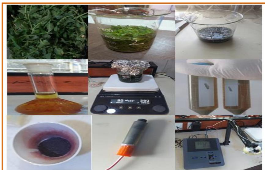
**Figure 1:** Preparation of nano substance and electrode construction.
